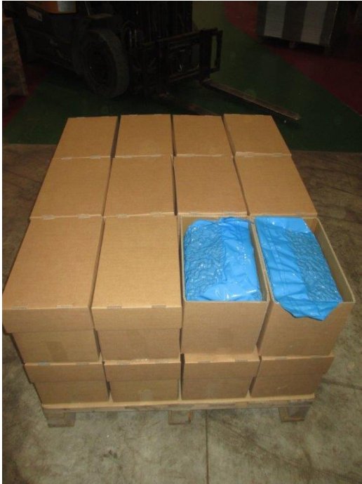
Partial view of 25 lb box on the pallet (bag in box, individual cover) 84 boxes per pallet
