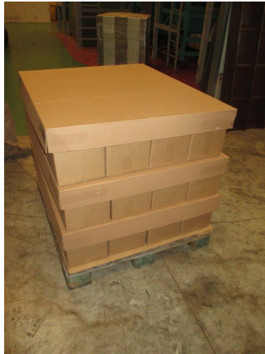
Partial view of 25 lb box on the pallet (bag in box, layer cover)
